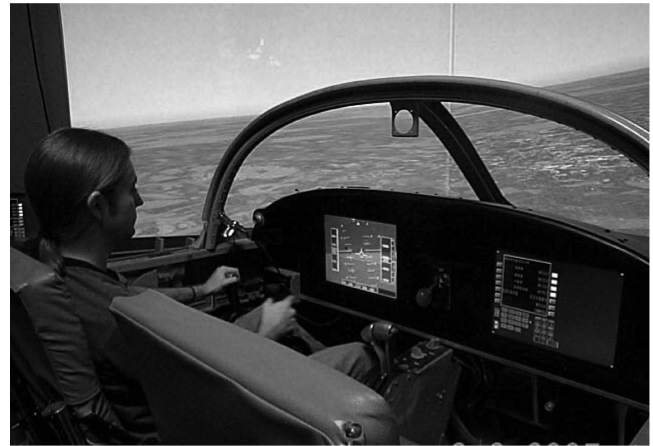
Fig. 5 Engineering flight simulator cockpit showing head-down displays and three-screen egocentric view.
